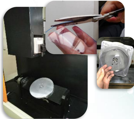
Knowledge-based 5-axis Plus-sized Bra Cup Plastic Shot Laser Cutting System
